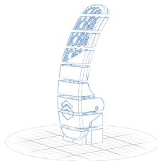
Part is digitally sliced into thin 2D layers
