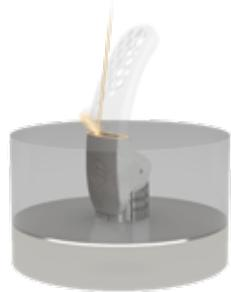
The laser melts a layer of powder for each 2D slice
